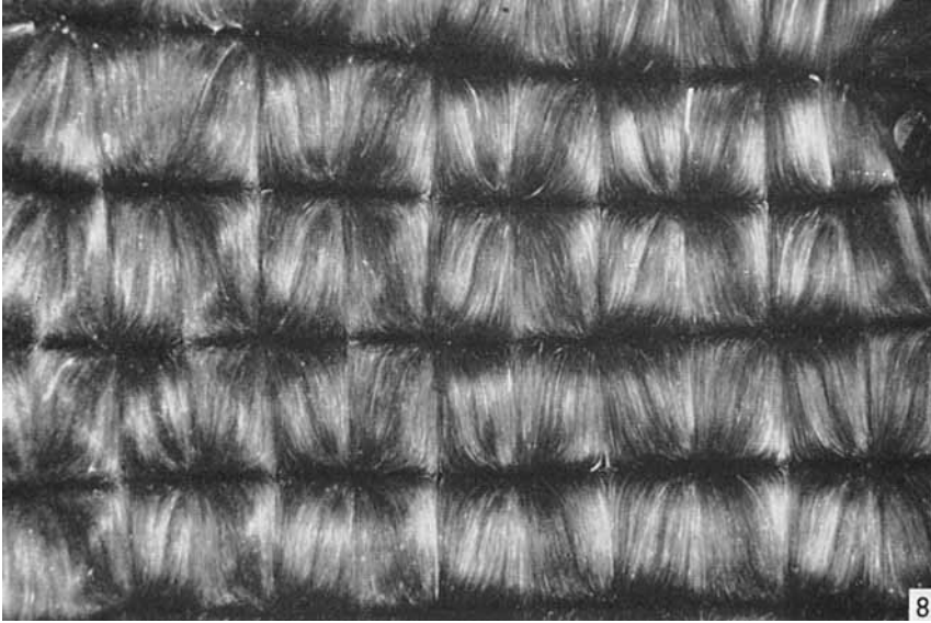
FIGURE 8. Photograph of bimodal convection at R = 25 \times 10^3 in an experiment by G. E. Willis. The convection layer contains silicone oil with Pr = 450 and is covered by a glass plate.
